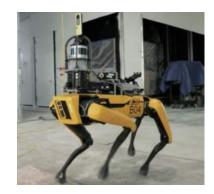
How is it making an impact? HoloBuilder launched a new application designed to work with partner Boston Dynamics autonomous Spot robots. The SpotWalk application can allow one of the robots to autonomously follow a path through a jobsite, collecting scans and 360-degree photos along the way at prescribed intervals. Further reducing the time and manpower allocated toward site progress documentation, the autonomous system has particular applications in challenging or hazardous construction sites.
